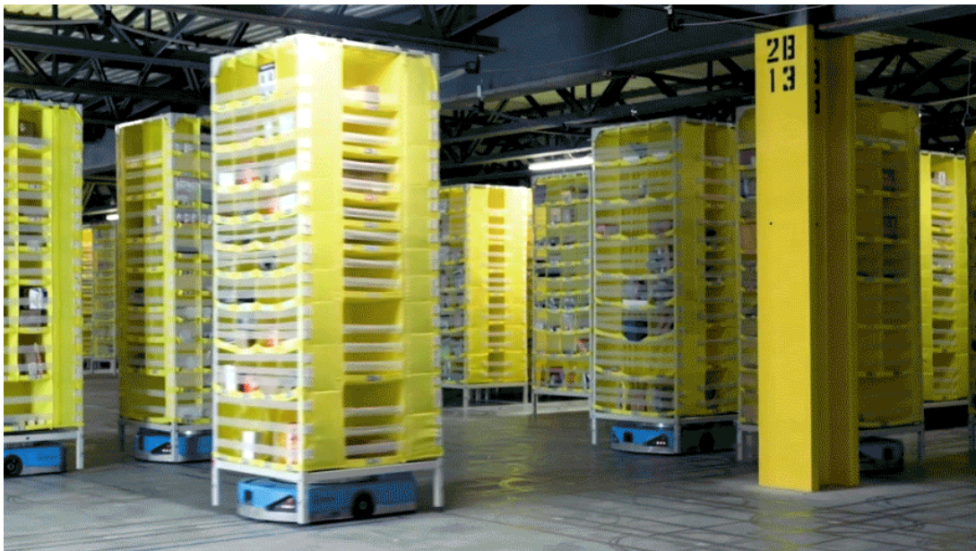
Figure 21: Amazon has a huge fleet of robots that automate its warehouses. This is an example of the Hercules robot that retrieves shelves of products and delivers them to employees, who then pick the items customers ordered for shipping (Amazon, 2023).
