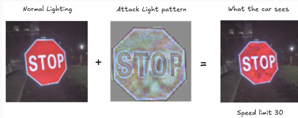
Figure 21: We don't need to even have physical access to objects. Just by shining the patterns as light on the objects, we can cause misclassifications and unintended behavior ( Gnanasambandam et al, 2021 ).
