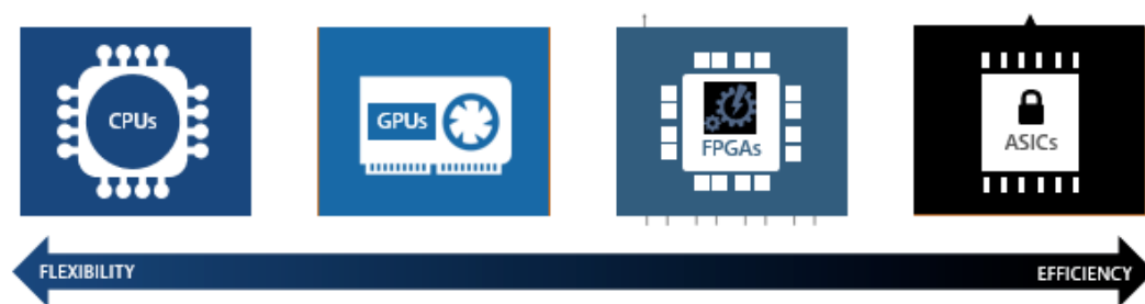
Figure 12: The spectrum of chip architectures with trade-offs in regards to efficiency and flexibility.
