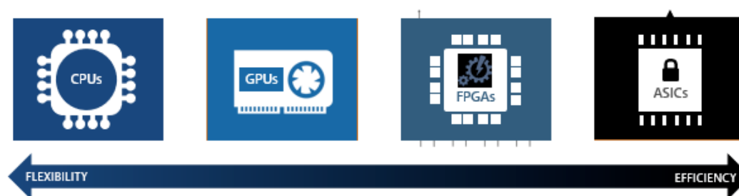
Figure 10: The spectrum of chip architectures with trade-offs in regards to efficiency and flexibility.
